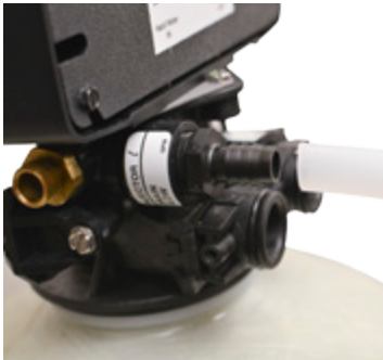
← 3.) Insert the backwash line onto the barb. It will be a snug fit. You will have to use a little force to get it all the way on. →
