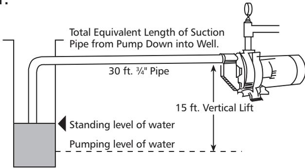
Pump Capacity 6 GPM
