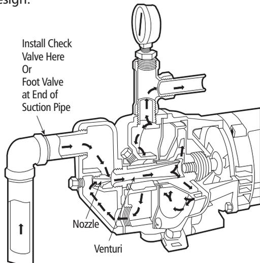
In shallow well jet pumps the jet assembly is built into the pump casing as in the Goulds Pumps J5S. Or, the jet assembly, shallow well adapters, can be bolted to the centrifugal pump. In either case there is only one pipe extending into the well . . . the suction pipe.
