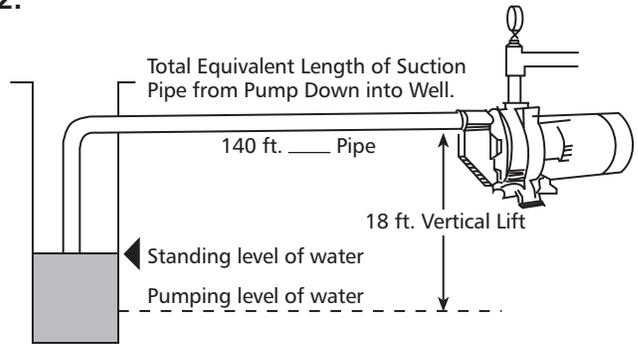
Pump Capacity 10 GPM
