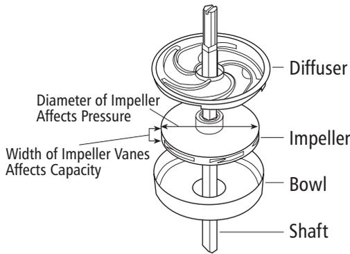
The capacity of a multistage centrifugal pump (submersible) is largely determined by the width of the impeller and diffuser, regardless of the number of stages. The pressure is determined by the diameter of the impeller, the speed at which it rotates and the number of impellers. The diameter is limited to the size of wells drilled. Most submersibles are designed to fit in four or six inch wells (or larger).
