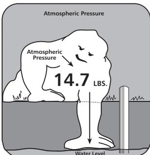
equal to about 14.7 lbs. per square inch at sea level. When the pressure of atmosphere is removed from inside of a pump the resulting condition is a vacuum or partial vacuum. It is also called suction.
