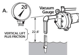
A reading of 20" on a vacuum gauge placed on a suction side of the pump would tell you that you had a vacuum or suction lift of 22.6 ft.
