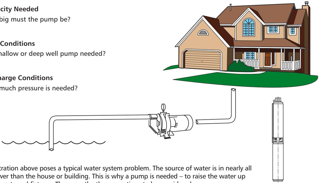
The illustration above poses a typical water system problem. The source of water is in nearly all cases lower than the house or building. This is why a pump is needed – to raise the water up to the faucets and fixtures. These are the three questions to be considered:
