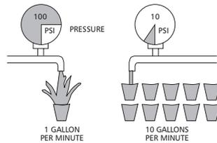
Now as to the resistance to flow which will be encountered, there are three causes. These are (1) the resistance by the outlet itself such as a partially rusted shower head, (2) friction loss in pipe lines, and (3) that resistance due to difference in elevations.
