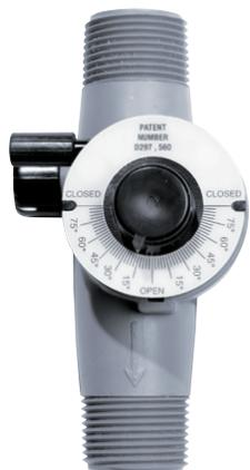
The Pentair® Wellmate® Micronizer installs easily to any hydropneumatic tank, drawing air into the water line through the air inlet. When properly installed and adjusted, the Wellmate Micronizer by Pentair will continually charge the tank with air for 30% to 50% of the pump's run time. Excess air is relieved through an Air Volume Control assembly installed in the tank.
