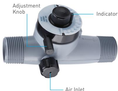
The pointer on the dial indicates that the micronizer is fully open when it is in line with the plumbing (12 o'clock position). This will give the least amount of air draw.
