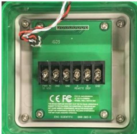
7 – Route the wires opposite the hinge and close the unit so that the wires come through the opening.
