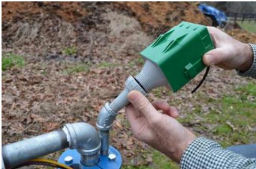
4 – Open the well watch to expose the electrical terminals by squeezing the locking tabs on the side of the unit.
