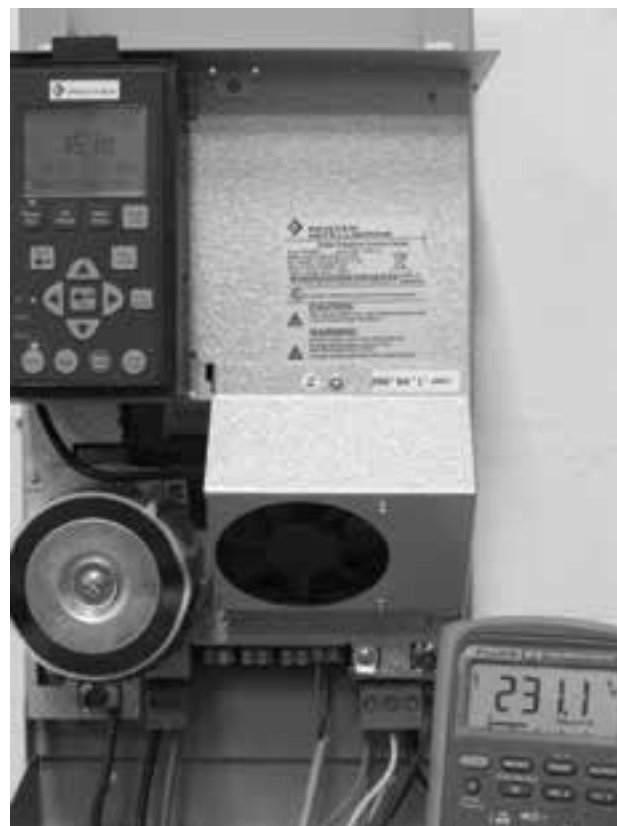
Figure 19. 45Hz voltage measurement w/out LPF
