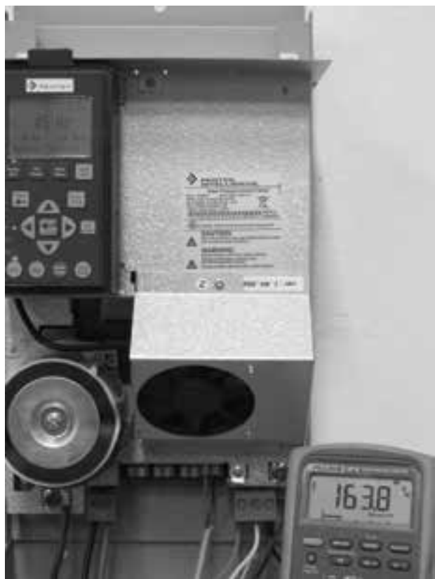
Figure 18. 45Hz voltage measurement w/ LPF
