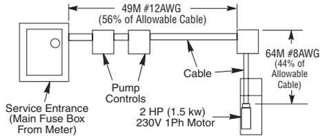
1. According to *Table IX*, a total of 87m of #12AWG cable is allowed to power the 2 HP motor. The percent of this total that has been used by the 49m of cable in the buried run is:  $49m / 87m = .56 = 56\%$ .
