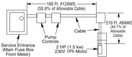
1. According to *Table VIII*, a total of 286' of #12AWG cable is allowed to power the 2 HP motor. The percent of this total that has been used by the 160' of cable in the buried run is:  $160' / 286' = .559 = 55.9\%$ .
